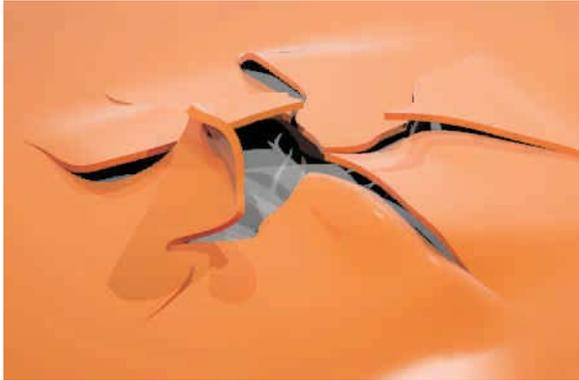
**Description:** Usually occurs around edges, trim, or hardware. Paint film not adhering to the substrate, or, layers of paint film separating.
