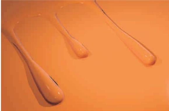
**Description:** Usually occurs on vertical surfaces. A heavy paint film collects and moves downward, setting in ripples.
