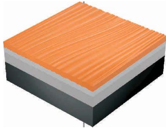
**Description:** Usually occurs when painting over repair work. Sanding scratches in the previous layer swell through the paint film.
