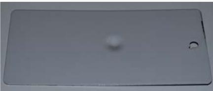
This test measures the products ability to 'absorb' punishment from flying debris, such as a dropped wrench. The higher the number, the better the flexibility.
