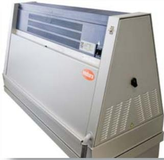
This test creates an artificial environment which tests for loss of gloss. In real terms .....5 years in operation with chemical washing, spillage and sunlight exposure will give you some quantitative results.
