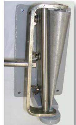
A steel panel is coated with a uniform thickness of the coating and is allowed to cure. The panel is then bent with a mandrel into a conical shape. The mandrel bend test measures the flexibility of the attached coating and its resistance to cracking when elongated. The test is measured at the point where there is no loss of adhesion or cracking.
