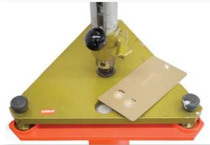
A test panel is coated with a uniform thickness of paint and allowed to cure. A standard weight is dropped onto the surface from varying heights, to test the impact resistance of the coating. The test can be performed with the paint side facing up (direct impact) or with the paint side facing down (reverse impact).
